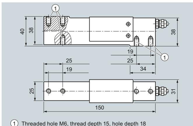
① Threaded hole M6, thread depth 15, hole depth 18
